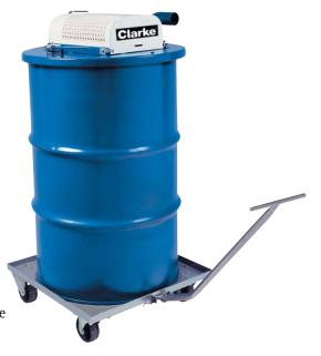
Air pressure passes through twin jet venturi to create a powerful vacuum. Despite its high air pressure, the noise level remains less than 79 decibels – lower than OSHA requirements. Equipped with a removable filter, the DWD air vacuum can handle wet or dry pickup, including sludge, sand, metal chips or more – an excellent alternative to traditional tank vacuums.
